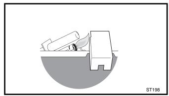
Fig. 32 Correct pilot flame appearance. OP pilot.
